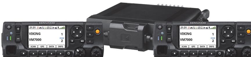
**Note** All heads are shipped from factory set as primaries. One of the heads must be programmed as a secondary to function correctly. Please refer to [Section 2.3.3](#).
