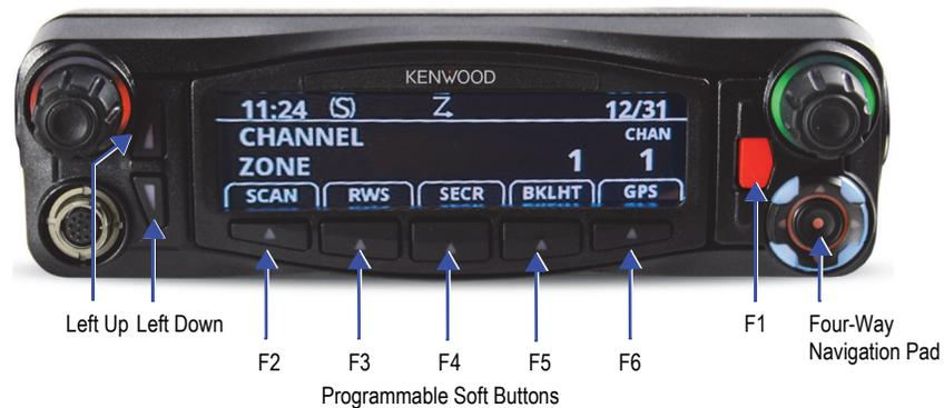
**Four-Way Navigation Pad** - This button pad is used to navigate through various radio functions and menus. The left and right buttons of the pad can be programmed with different radio functions.
